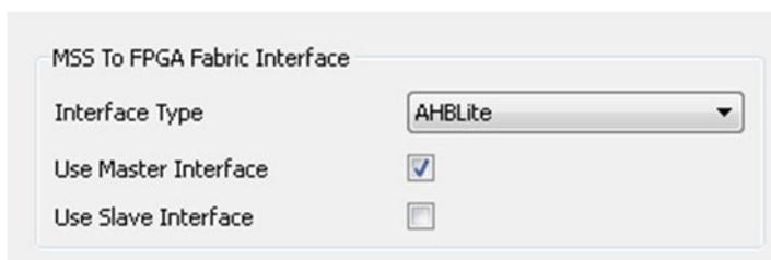
**Figure 1-1 • MSS to FPGA Fabric Interface Core**
