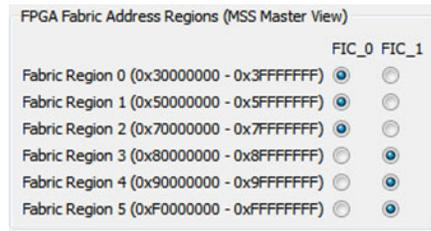
**Figure 1-3 • FPGA Fabric Address Regions (MSS Master View)**
