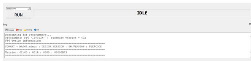
Figure 7-9. Programmer 138013A Showing Design Version 001A On Successful Update
