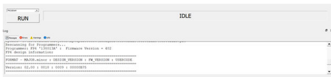
Figure 7-7. Programmer Connected With Design Version 0018
