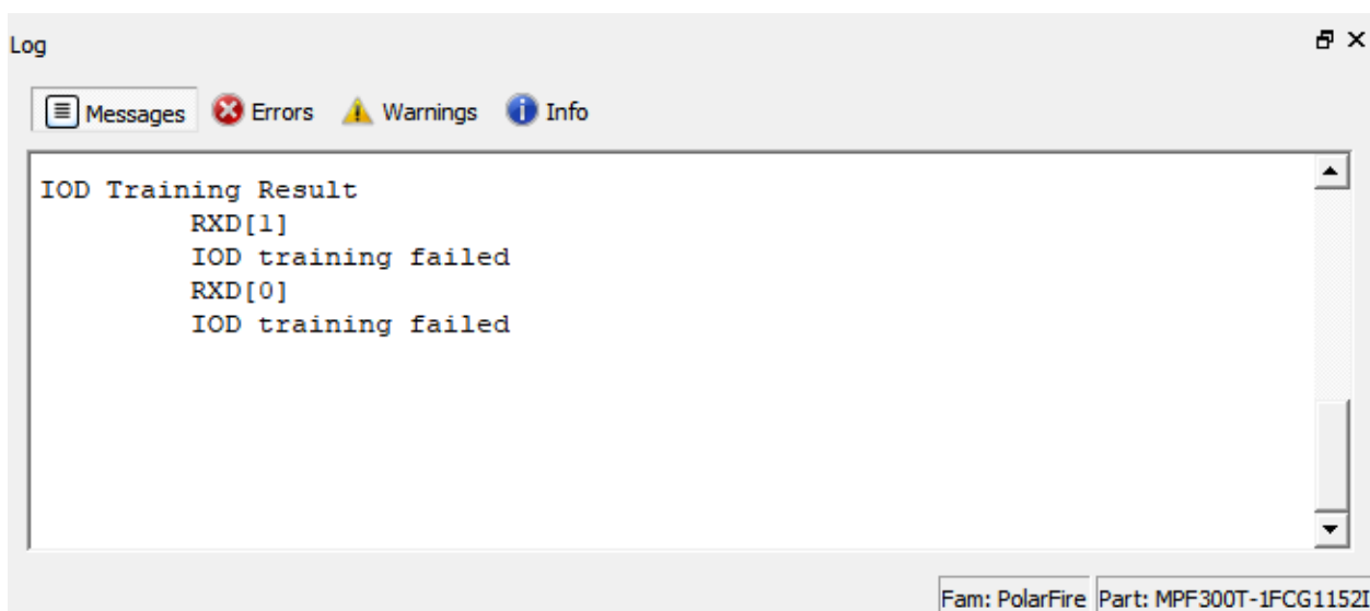
Figure 3-90. SmartDebug Log Window—Training Failed
