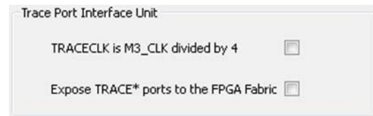
Figure 1-5 • TPIU FPGA Fabric Interface Configuration
