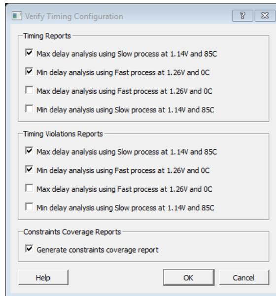
Figure 6: Verify Timing Configuration Options Dialog Box
